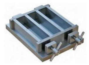
Small cube molds may be useful for assessing only compressive strength, the standard 50 mm cube mold being used for this purpose.
