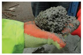
to dry out; this prevents adequate compaction and correct hydration of the cement so that that a weak laying course is produced and rapid failure occurs.
